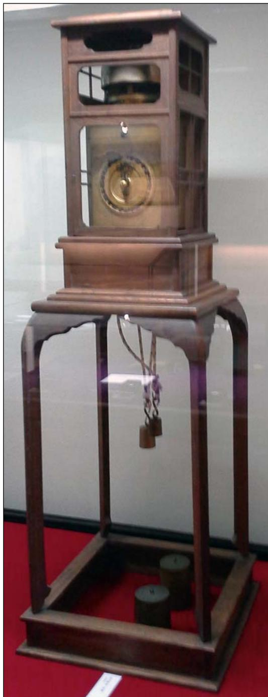
**Figure 7, left.** Early weight-driven Japanese clock with foliot escapement.
