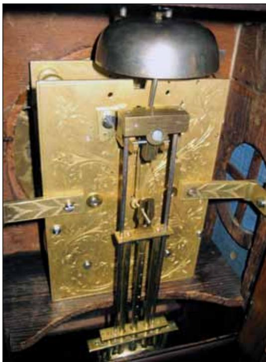
**Figure 3.** Rear view showing the engraved backplate and pendulum.
