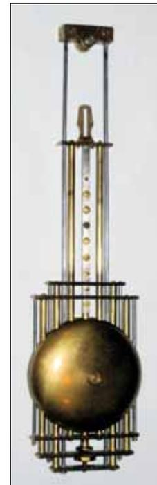
**Figure 4.** Gridiron pendulum with “tin whistle” adjuster.
