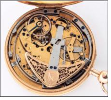
Self-winding (or "automatic") watches are nothing new. This one is circa 1810 and is signed "Breguet a Paris," but the company recently stated that the watch is rare and interesting but "not a timepiece manufactured by the Breguet workshops." Assuming that the watch is moved regularly, its pedometerstyle weight will keep the movement wound and ticking for the new owner who paid \$11,250.
