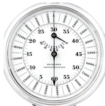
Figure 6. Seikoshia made this ca. 1940 phototelemeter for the Japanese navy. It timed the distance of artillery shell firings, comparing the flash and boom. An original fitted wood case with appropriate Japanese script was included. Estimate $300/400; sold for $600. COURTESY OF WILLIS HENRY AUCTIONS.
