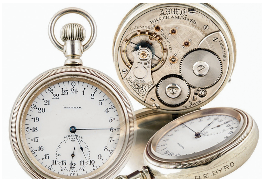
Figure 5. There was more than one sidereal pocket watch in the sale. Rare and useful in navigation, these timepieces reference stars rather than the sun for timing the earth's rotation, resulting in a day roughly four minutes shorter than regular 24-hour timekeeping. This ca. 1913 high-grade Model 92 by Waltham Watch Co., with 24-hour dial, has "R.E. Byrd" engraved on its edge. Even without Admiral Byrd's name, its selling price was justified and, unusually, below expectations. Estimate $3000/3500; sold for $2400. COURTESY OF WILLIS HENRY AUCTIONS.
