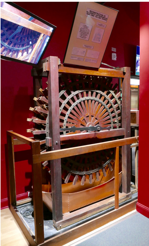
Twentieth-century full-scale replica of the circa 1356 Richard of Wallingford clock.
