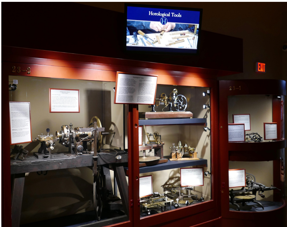
Horological tools including, on the left, a rose engine from the workshop of A.I. Breguet.
