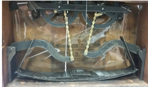
Before the Connecticut clock factories mastered the manufacturing of coiled springs, other methods were attempted to replace hanging weights. Inside the case of a Birge & Fuller steeple clock were these "wagon springs." Disaster strikes when those little chains break during winding, meaning that many of these cases have replaced glass tablets. This clock sold for $3998. Frishman photo.
