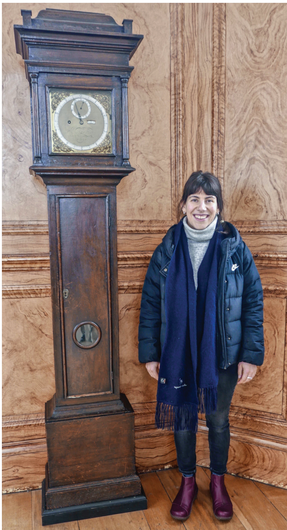
Figure 5. Daniela Corda every week winds the circa 1691 Thomas Tompion “Sideral Angle Clock” at the Royal Observatory Greenwich. Designed by the first Astronomer Royal, John Flamsteed, the clock indicates time based on the Earth’s angular rotation.
